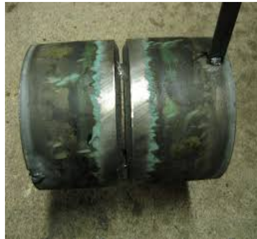
Measure scribe lines, weld fillet.
