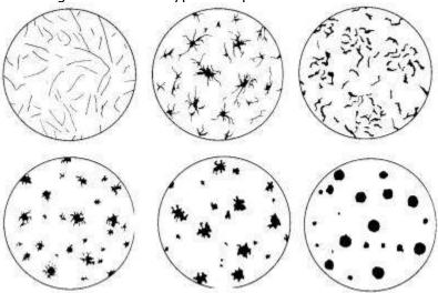
These types may be identified manually or automatically. MiC graphite morphology detection engine can isolate any of these with subclasses.
