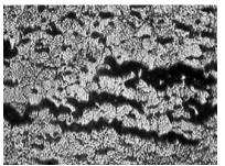
In present case the failure of tube seems to have occurred due to long term over- heating, above
