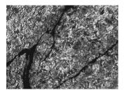
TCR Engineering Services concluded that the shaft failed due to pre-existed Heat treatment cracks under operational load.
